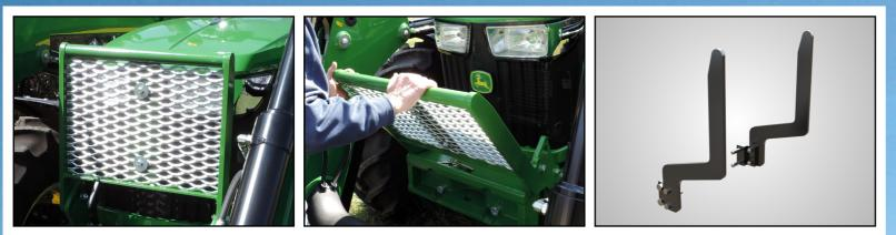
**Guard Options:** Protect the front of your investment with a grille guard or bump guard. The fold down grille guard, provides a more compact and functional design.
