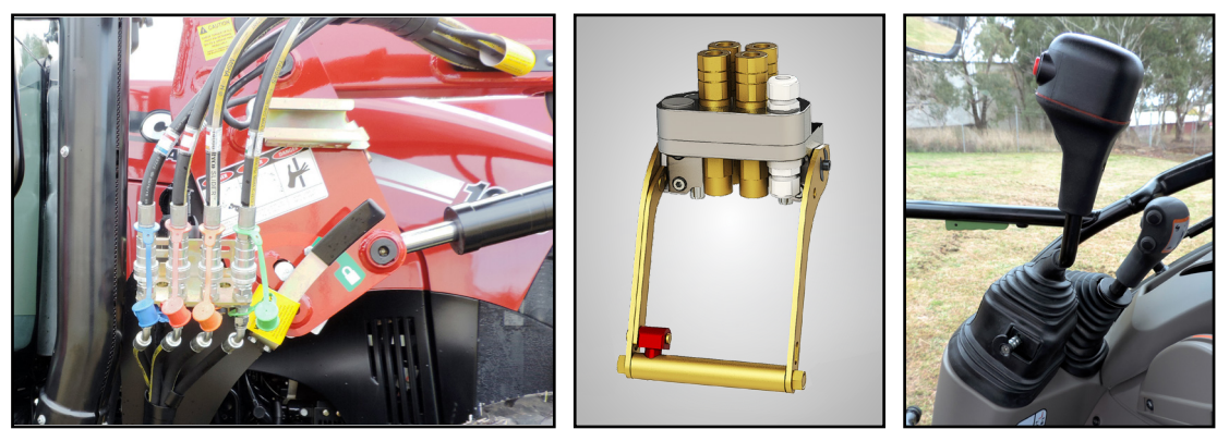
Midmount Remotes Kit: Integrated loader controls utilising host tractor joystick conveniently positioned in the existing control console.
