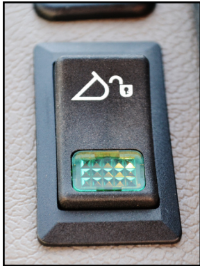
Electric Diverter Valve Kit: Switch between the rear control or the loader control from within the cabin, with a press of a button, increasing your productivity.
