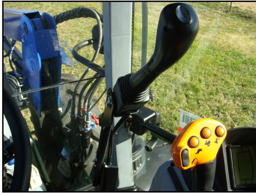
Auxiliary Valve Kit: Multi-position joystick control to suit individual operator requirements. Loader connection is easy with a multi-coupler.
