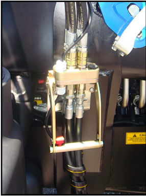
Midmount Remotes Kit: Integrated loader controls utilising host tractor joystick conveniently positioned in the existing control console.
