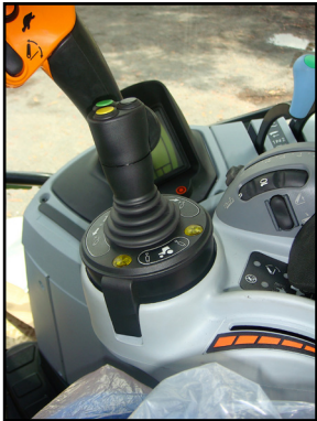
Electric Diverter Valve Kit: Switch between the rear control or the loader control from within the cabin, with a press of a button, increasing your productivity.
