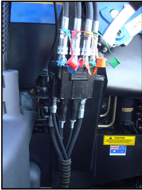
Auxiliary Valve Kit: Multi-position joystick control to suit individual operator requirements. Loader connection is easy with a multi-coupler.
