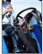
**Auxiliary Valve Kit:** Multi-position joystick control to suit individual operator requirements.
