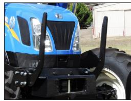
**Guard Options:** Protect the front of your investment with a grille guard or bump guard. The grille can be removed for night work.
