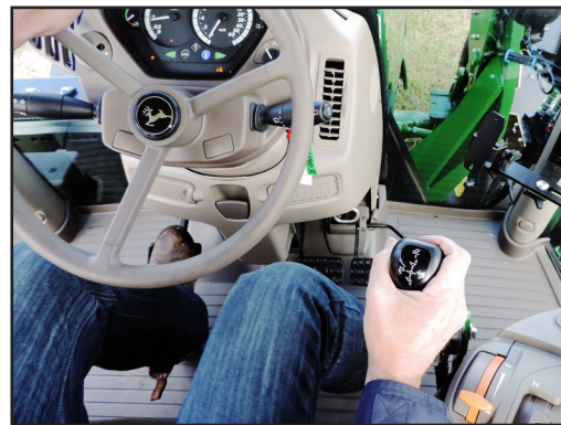
Auxiliary Valve Kit: Multi-position joystick control to suit individual operator requirements and compatible with a swivel seat.
