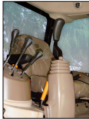
Midmount Remotes Kit: Integrated loader controls utilising host tractor joystick conveniently positioned.
