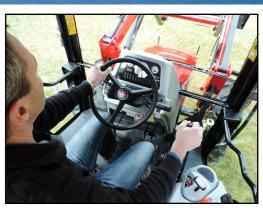
**Auxiliary Valve Kit:** Adjustable joystick control to suit individual operator requirements. Loader connection is easy with a multi-coupler.
