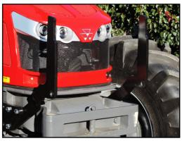
**Guard Options:** Protect the front of your investment with a grille guard or bump guard. The fold down grille guard, provides a more compact and functional design giving you access to all serviceable components of the tractor. The grille can be removed for night work.
