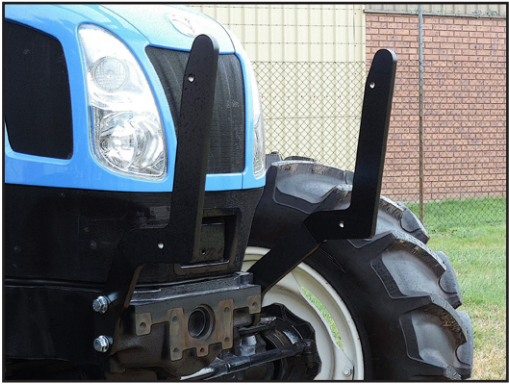
Guard Options: Protect the front of your investment with a grille guard or bump guard. The grille can be removed for night work.
