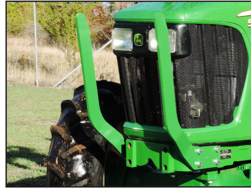
Guard Options: Protect the front of your investment with a grille guard or bump guard.
