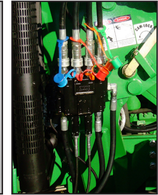
Auxiliary Valve Kit: Multi-position joystick control to suit individual operator requirements. Multi-coupler optional.
