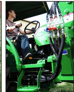
Midmount Remotes Kit: Integrated loader controls utilising host tractor joystick conveniently positioned in the existing control console.
