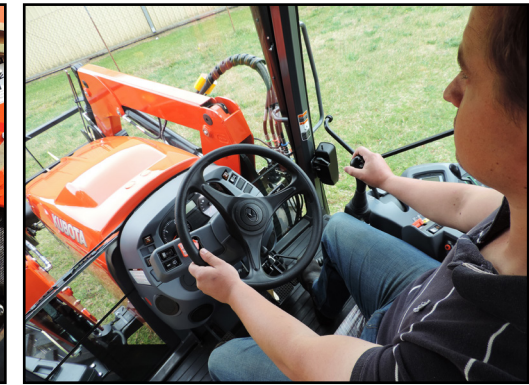
Auxiliary Valve Kit: Adjustable joystick control to suit individual operator requirements.
