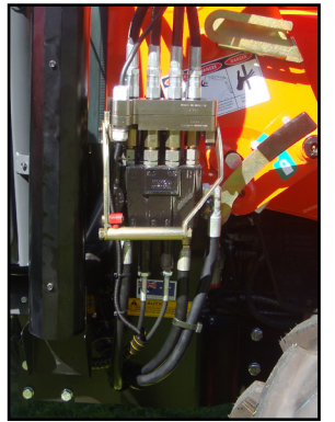
Auxiliary Valve Kit: Adjustable joystick control to suit individual operator requirements.
