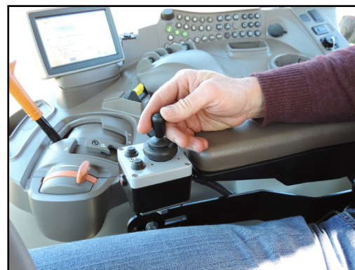
Auxiliary Valve Kit: Electric joystick control positioned to suit operator requirements. Loader connection is easy with a multi-coupler.
