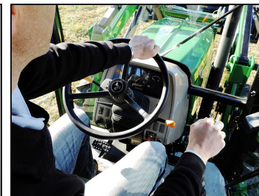
Midmount Remotes Kit: Integrated loader controls utilising host tractor joystick conveniently positioned in the existing control console.
