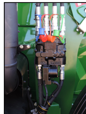
Auxiliary Valve Kit: Electric joystick control positioned to suit operator requirements. Loader connection is easy with a multi-coupler.
