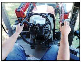
**Auxiliary Valve Kit:** Multi-position joystick control to suit individual operator requirements. Loader connection is easy with a multi-coupler.
