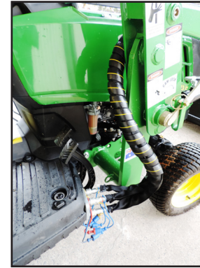
Midmount Remotes Kit: Integrated loader controls utilising host tractor joystick.
