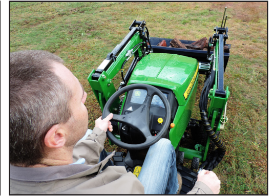
Midmount Remotes Kit: Integrated loader controls utilising host tractor joystick.
