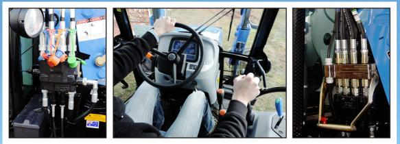
**Auxiliary Valve Kit:** Console integrated joystick control to suit operator requirements. Loader connection is easy with a multi-coupler.
