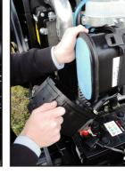
**Service Access:** Easy access to all the serviceable parts and components of your tractor, including air filters, oil filters and sump plug.
