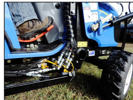
Midmount Remotes Kit: Integrated loader controls utilising host tractor joystick.
