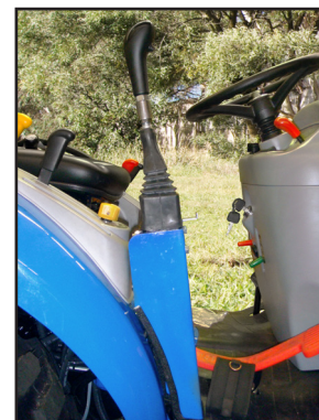
Midmount Remotes Kit: Integrated loader controls utilising host tractor joystick.
