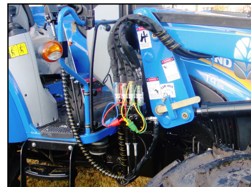
Auxiliary Valve Kit: Multi-position joystick control to suit individual operator requirements.
