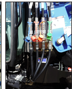
Midmount Remotes Kit: Integrated loader controls utilising host tractor joystick. Loader connection is easy with a multi-coupler.
