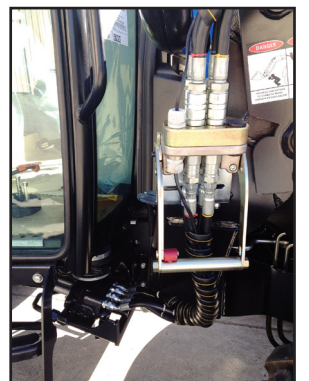
Midmount Remotes Kit: Integrated loader controls utilising host tractor joystick. Loader connection is easy with a multi-coupler.
