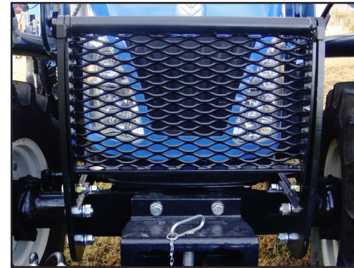
Guard Options: Protect the front of your investment with a grille guard or bump guard. The fold down grille guard insert creates a more compact and functional design.
