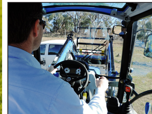
Midmount Remotes Kit: Integrated loader controls utilising host tractor joystick. Loader connection is easy with a multi-coupler.
