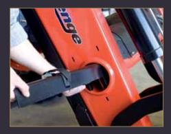
After usage, the safety lock fits neatly back into the loader cross bar. Challenge decided to use mechanical safety locks rather than hydraulic taps as a hydraulic fitting can be undone while an operator is under the loader area. The use of mechanical safety locks ensures the loader can never be lowered while the mechanical lock is in place.
