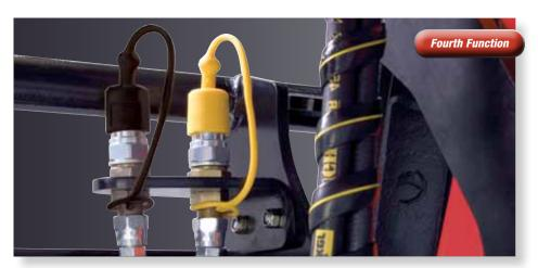
Along with the included third function service, an optional fourth function service is available to be fitted at the time the loader is ordered. It can also be purchased as an after-market fitment, with standard couplings or an easy-to-use multi-coupling system. The third and fourth function services are activated right from the loader joystick.
