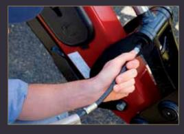
All pins have easy access greasing-points. By regularly greasing your CLX<sup>TM</sup> front-end loader, you will ensure your loader remains in good working order. Although the bearings are selflubricating, it is important to keep fresh grease in the bearings for best operational performance.
