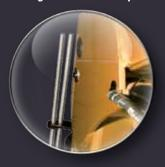
5. The implement level gauge has been made from solid steel bars and a welded cast steel bracket to ensure the strength of this feature. The level gauge is mounted on the inside of the loader below the level of the frame arm for ease of sight and protection.
