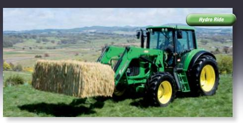
Travelling with or without a load, the all new CLX<sup>TM</sup> Hydro Ride system will sense and adjust to the current pay load being carried. While travelling from point A to B, you can enjoy the smoothest ride possible with this new system. The CLX<sup>TM</sup> Hydro Ride system can be turned on or off from the loader joystick controls, making it convenient when loading and stacking where more precision is needed.
