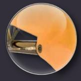
2. Flush pin design and hidden hydraulic hoses increases loader to tractor clearances and provides clean boom arm surfaces free from hoses, brackets, fittings and other components traditionally mounted on the boom arm surface.
