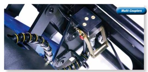
All loaders are designed to allow the use of multi-couplers to increase operator ease of use when changing third & fourth function dependent implements from quick couplers. Challenge Implements also offer multi couplers on  $CLX^{TM}$  loaders for easier hydraulic coupling of the loader, on and off the host tractor.
